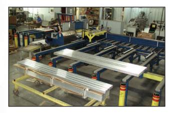
Four twin-head CNC production saws – very versatile in processing high volume and specialty cuts. Our smaller manual saws are highly advantageous for specialty angles, more flexible on materials and specialty parts. The automatic B & O Bundle Cut saw processes bundled material at precision tolerances (+/- .005") with a cut window of up to 12"x36" and a 36" blade. This saw can cut, be loaded and unloaded simultaneously.
