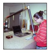
Quality control is maintained by our in-house lab to ISO 9001:2008 certification standards. Inspections are preformed on incoming extrusions, 1st piece and in-process parts, via Micro-Vu (Video Optical Comparator) various gauges and calipers. Reverse engineering, calibrations, close tolerance inspections and automated inspections are carried out on coordinate measuring machines.
